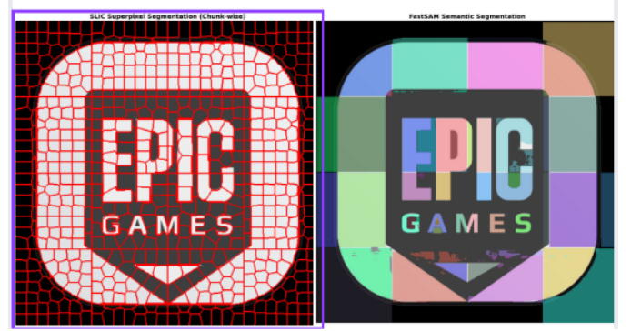
Fig. 2: Comparison of SLIC and FastSAM segmentation on sample image showing semantic region boundaries
